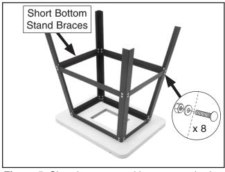
Figure 5. Short bottom stand braces attached to the legs.
